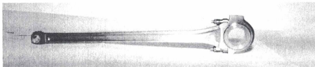
The distinctive Gresley inside connecting rod; it could be for real!
