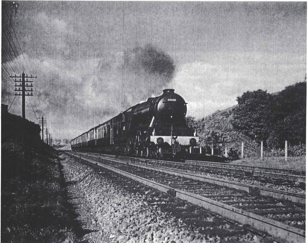
Another great shot by H. K. Harman. This one is from a much later era, 1959, and at a location further north at the famous Cockburnspath bank. 60080 DICK TURPIN recently fitted with the Kylchap double chimney looks in fine fettle as she storms up the bank, with not the slightest problem of drifting exhaust.
